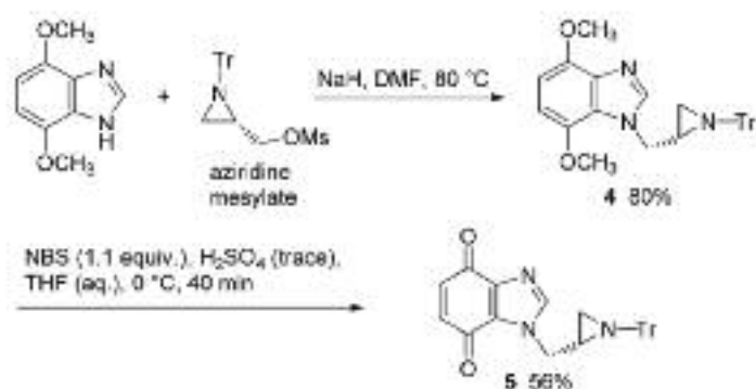
Scheme 2. Synthesis of N -[(aziridin-2S-yl)methyl]benzimidazolequinone.
