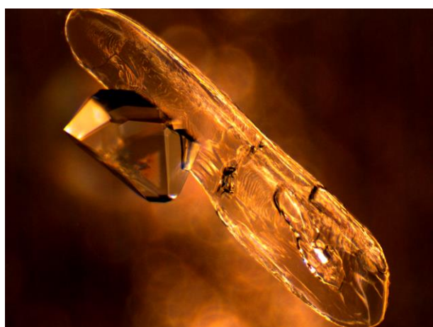
Figure 1. Metastable Form II Piracetam (rough dissolving crystal) undergoing a solution mediated polymorphic transformation to FIII (smooth growing crystal ).
