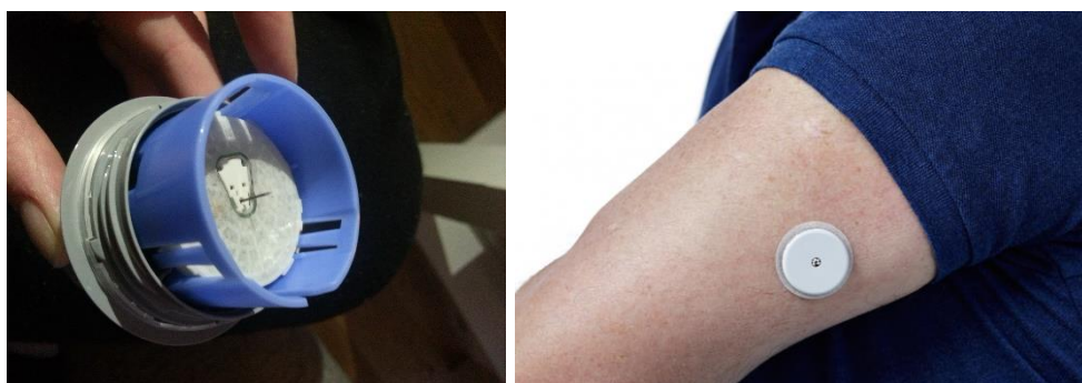
Fig. 3: The Abbott Libre applicator (left, [4]) showing the sampling fibre and (right,[5]) the glucose sensing patch on the upper arm after attachment.
