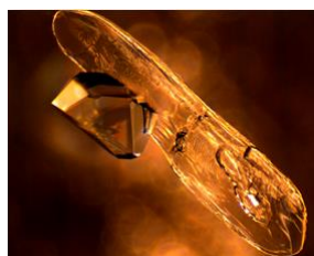
Optical Micrograph of a metastable Form II piracetam.
