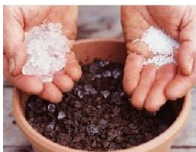
Fig. 2: Dry hydrogel (right) swells up (left) by absorbing water.
