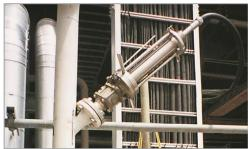
Figure 6. In process particle measurement instruments using focused beam reflectance measurement technology (see Appendix) implemented in lab and production settings
