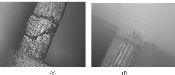
**Figure 1.0.** Laser-induced damage in an SU-8 microturbine blade, showing (a) 50  $\mu$ m-wide leading edge and (b) trailing edge of microturbine rotor (c) and (d). The leading edge has cracked during processing, and both edges show evidence of melting and reflow which will have induced stress.
