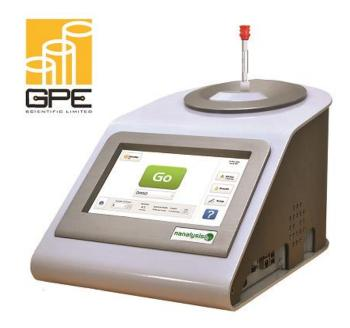
The machine offers good sensitivity and the high resolution allows spectra to be measured quickly. The data can be processed directly (even while wearing safety gloves) through the built-in resistive touchscreen without connecting an external computer.
