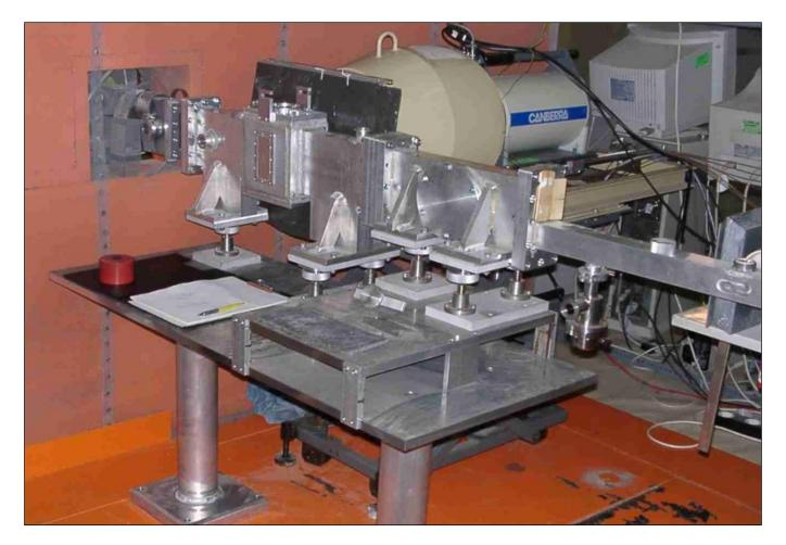
**Figure 1.1.** Prompt Gamma Activation Analysis station at the Institute of Isotopes, Budapest Research Reactor (BRR).
