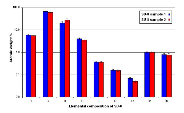
Figure 1.3. Atomic weight percentages of different elements in SU-8 samples 1 and 2, as determined by PGAA.
