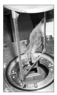
Figure 1.2. SU-8 microturbine sample fastened with Teflon strings onto an aluminium frame for introduction into the PGAA measurement chamber.
