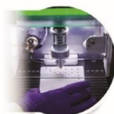
TLC/CMS – mass analysis of TLC spots
