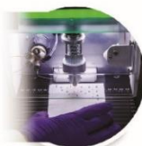
TLC/CMS - mass analysis of TLC spots
